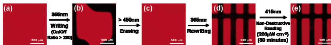
Figure 4. Microsized erasable ES IPT-fluorescence photoimaging on a spin-coated BP-BTE/DHBO-loaded PMMA film and its nondestructive readout capability; (a) initial open-form state; (b) writing; (c) erasing; (d) rewriting; and (e) continuous nondestructive reading under irradiation with the relatively high-intensity 415 nm light ( 200 \mu\text{W cm}^{-2} ) for 30 min. The dark region represents the irradiated area with the 365 nm UV light.
